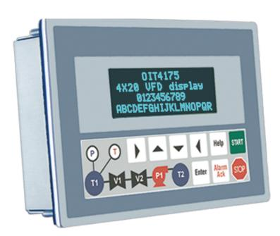
The OIT4175 has an alphanumeric vacuum fluorescent display and a membrane-style keypad with cusom slide in legend. Each key is programmable, allowing you to define a unique keypad to match your specific application. The legendable insert feature means you don't have to pay extra for custom overlays to achieve a custom look.
